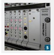
RAS 90 (PZB90) system consists of central device RAS90, locomotive balise, track balises and signalling and operating elements located in the locomotive cabin. The system offers high level of reliability and safety while maintaining the main idea of ALTPRO INDUSI based ATP systems - simplicity, robustness and longevity.
