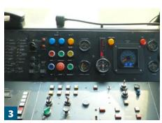
**AUTOSTOP (160)** system consists of central device **RAS8385**, locomotive balise, track balises and signalling and operating elements located in the locomotive cabin. It is a simple, robust and extremely reliable system. ALTPRO can offer any service/ product related to this system from project documentation all the way to system commisioning.
