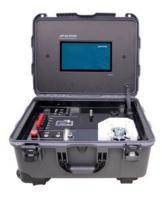
Testing device used for incremental encoder and pick up sensors testing. It is designed to be simple and easy to use for field testing activities.
