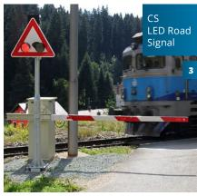
**RLC23 Level Crossing Protection** system is a 2 out of 2 SIL4 certified system. ALTPRO is producing all system components (central device, train detection, barriers and signals) which enables the Customer maximum flexibility. RLC23 is a highly configurable system and can be easily adapted to any requirement set by the Customer.
