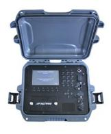
Testing device used for track balise control which is capable of generating short impulse while track balise is active (the rest of time test track balise) or inactive. The width of that impulse is proportional to the travel speed of the train.
